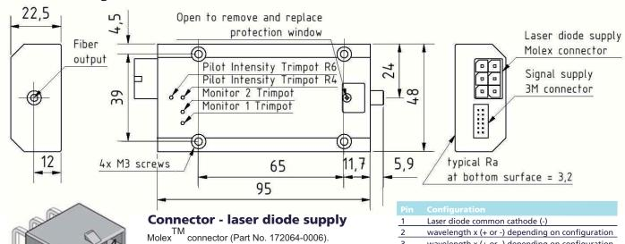
Pin connection dependant on individual electro-optical configuration. Maximum current per pin is 26 A if total current to cathode exceeds 26 A two pins must be connected to cathode of driver board Counterparts for external cable
