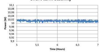
The graph below shows the power stability of the entire range of ALS-GR-532 lasers: short term fluctuations <+/-0.2% (limited by detector noise) and long term fluctuations <+/-0.3%.
