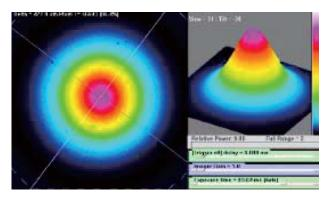
ALS-GR-532 lasers are based on only single mode fibers architecture, demonstrating an ultra-stable high quality single spatial mode.
