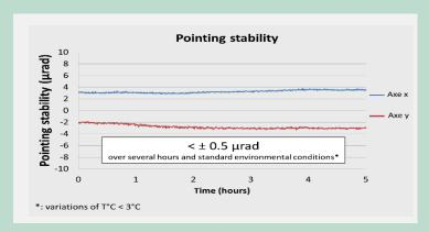
The graph shows the stability of pointing of a standard ALS-GR-532 lasers. Customers from industry validated our solution as the only one on the market to be able to replace and improve their performances performed with Argon lasers regarding the central frequency stability and the pointing stability.
