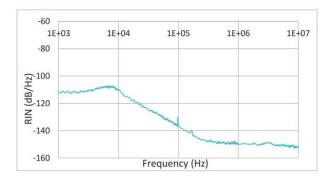
Below is a typical RIN data of an ALS IR fiber laser with internal laser seed <50kHz (typical 25 kHz). This spectrum is representative of the RIN level of the entire ALS IR range of lasers set up in constant power mode.
