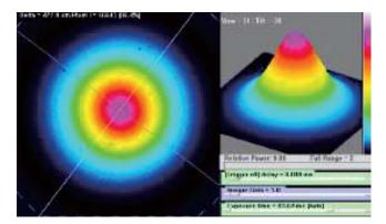
ALS lasers are based on only single mode fibers architecture and so offer an ultra-stable high quality single spatial mode. Typical value: M2 < 1.1 (typ. 1,05)
