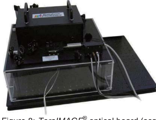
Figure 8: TeraIMAGE ® optical board (scanning range 50 mm x 50 mm).
