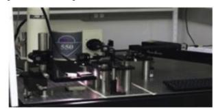
Testbed #1 is shown in the figure above. This laboratory based instrument was developed through ASTID, NSF and NAI funds. It has the same optical parameters as the Mars SHERLOC version including components (laser and CCD), spectrometer resolution, and photon budget that has been used to collect the data presented here. A flight like version of the instrument with form and fit identical to the 2020 version is currently undergoing testing.
