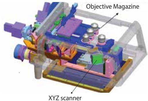
**Patented Objective Exchanger**
