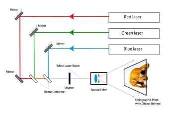
Figure 1: Typical white light holographic set-up
