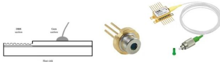
Fig. 1 Schematics of a DBR diode laser gain chip structure and examples of standard packages for DBR diode lasers
