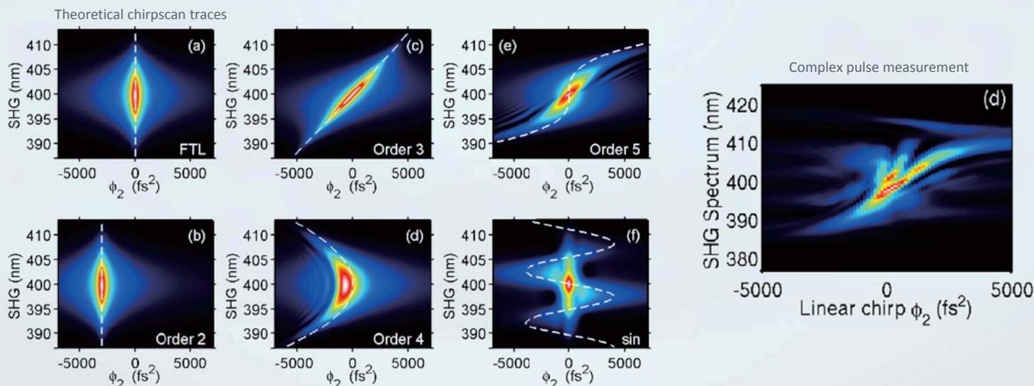
Data from V.Loriot et al: "Self-referenced characterization of femtosecond laser pulses by chirpscan" Optics Express 2013
