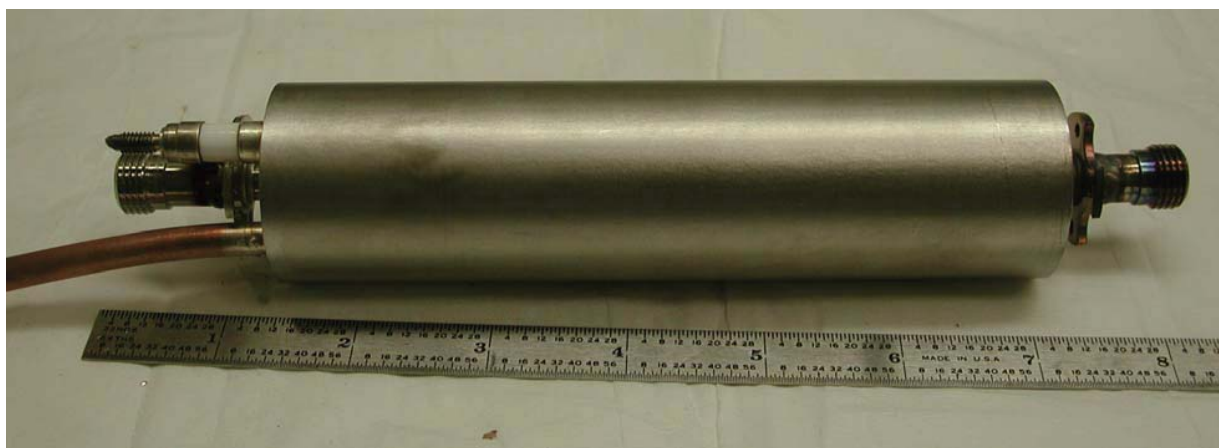
Photo of 9 inch, 248nm NeCu laser tube
