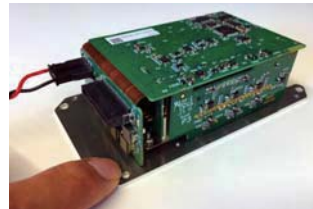
Hermetically sealed package with integrated electronics
